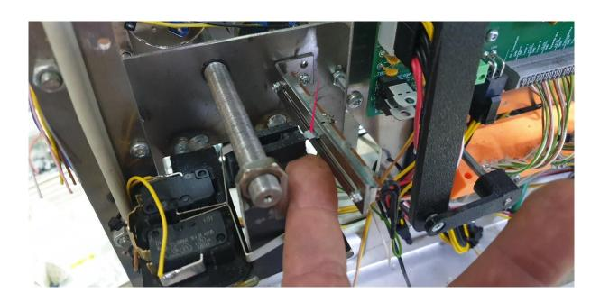
7. Now manually turn the trim wheel on the Captain's side until the small steel pendulum drops off the threaded shaft.
