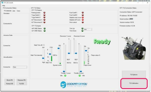
*9.* Now calibrate SpeedBrake, Rev 1, Rev 2 and Flaps in the order given. Bring the lever to the respective end position and click on the button. When you're done, click Done.
