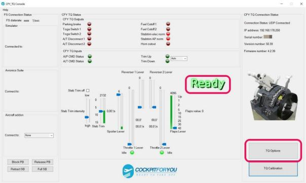
**13.** Please switch from UDP Connection to TCP Connection and click the "Done" button The CFY Console must then be restarted for this setting to take effect.
